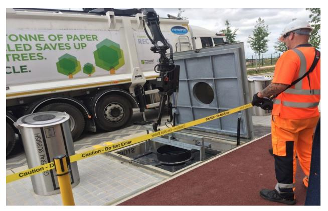
Fig 19 Underground bins hook-lift system in the ground
