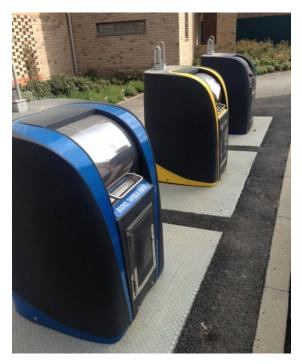
Fig 16 Single Hydraulic bring banks collecting mixed recycling
