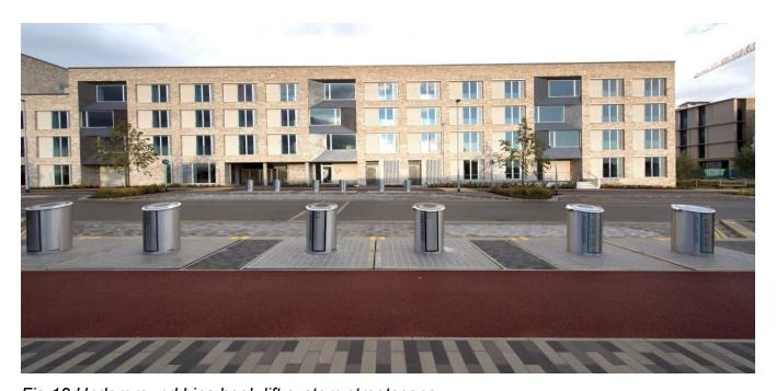
Fig 18 Underground bins hook-lift system streetscape
