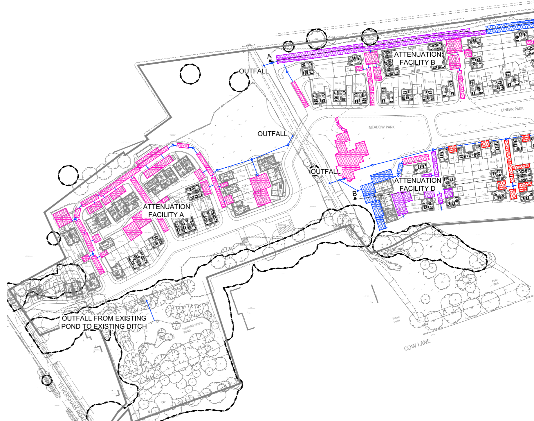
Figure 61. Drainage Strategy, Attenuation Crates
