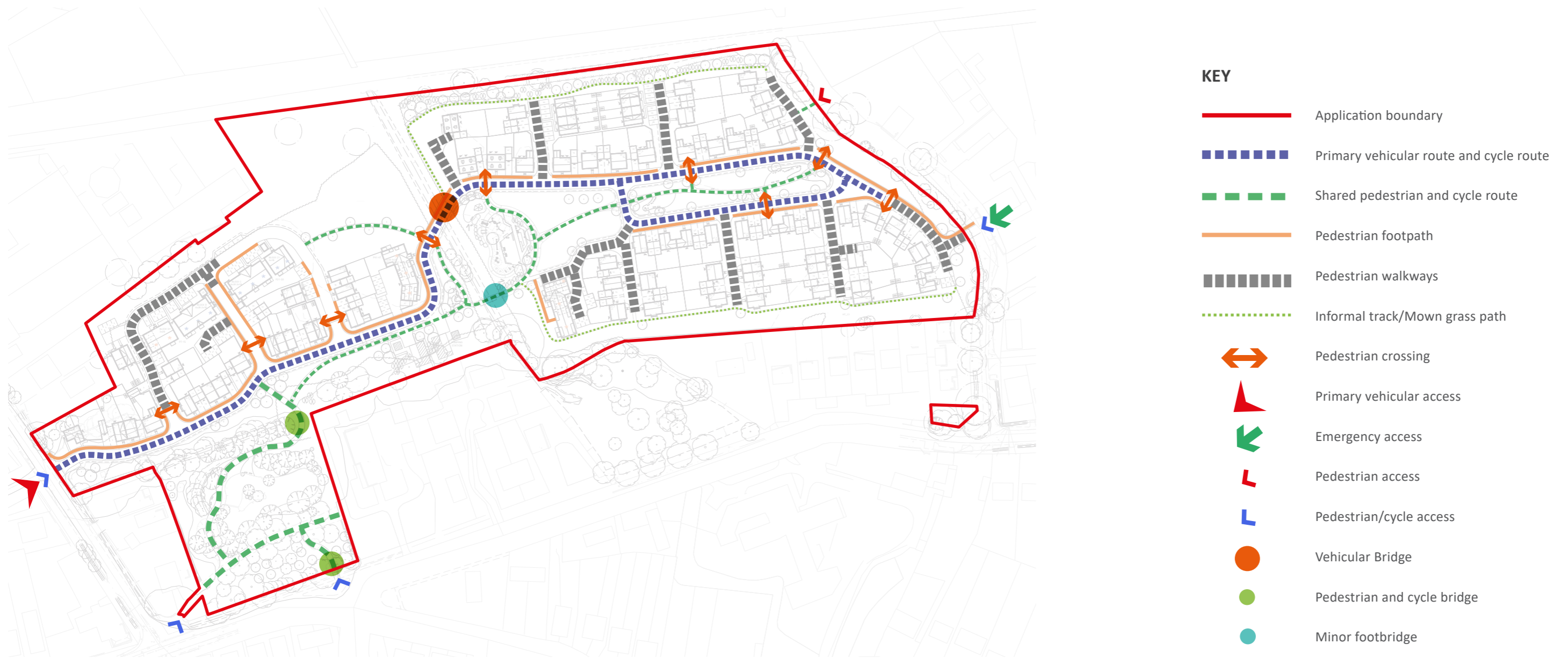
Figure 59. Pedestrian, Cycle Access and Circulation
