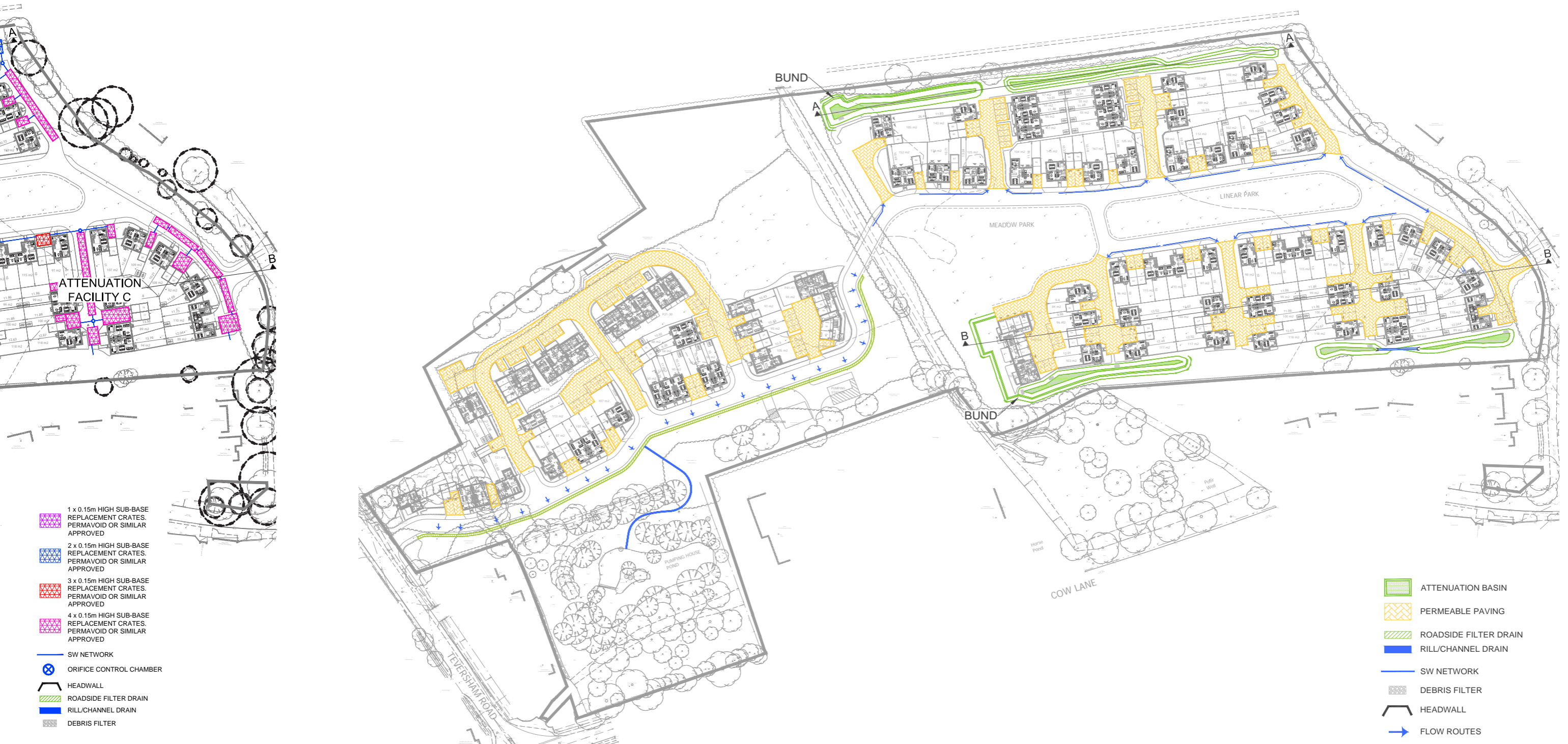
Figure 62. Drainage Strategy, Attenuation Basins and Permeable Paving
