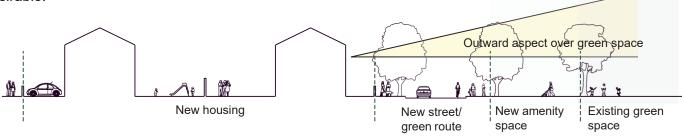
Fig 36 Section through indicative development illustrating green space consolidated into larger amenity space. This gives housing an outlook across the green, providing pleasant aspect and surveillance.
