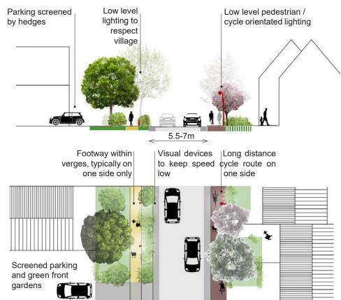
Fig. 28 - Appropriate layout for streets with through traffic
