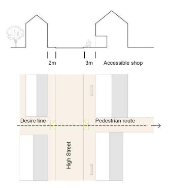
Fig 48 High Street section and plan illustrating measures for improved accessibility
