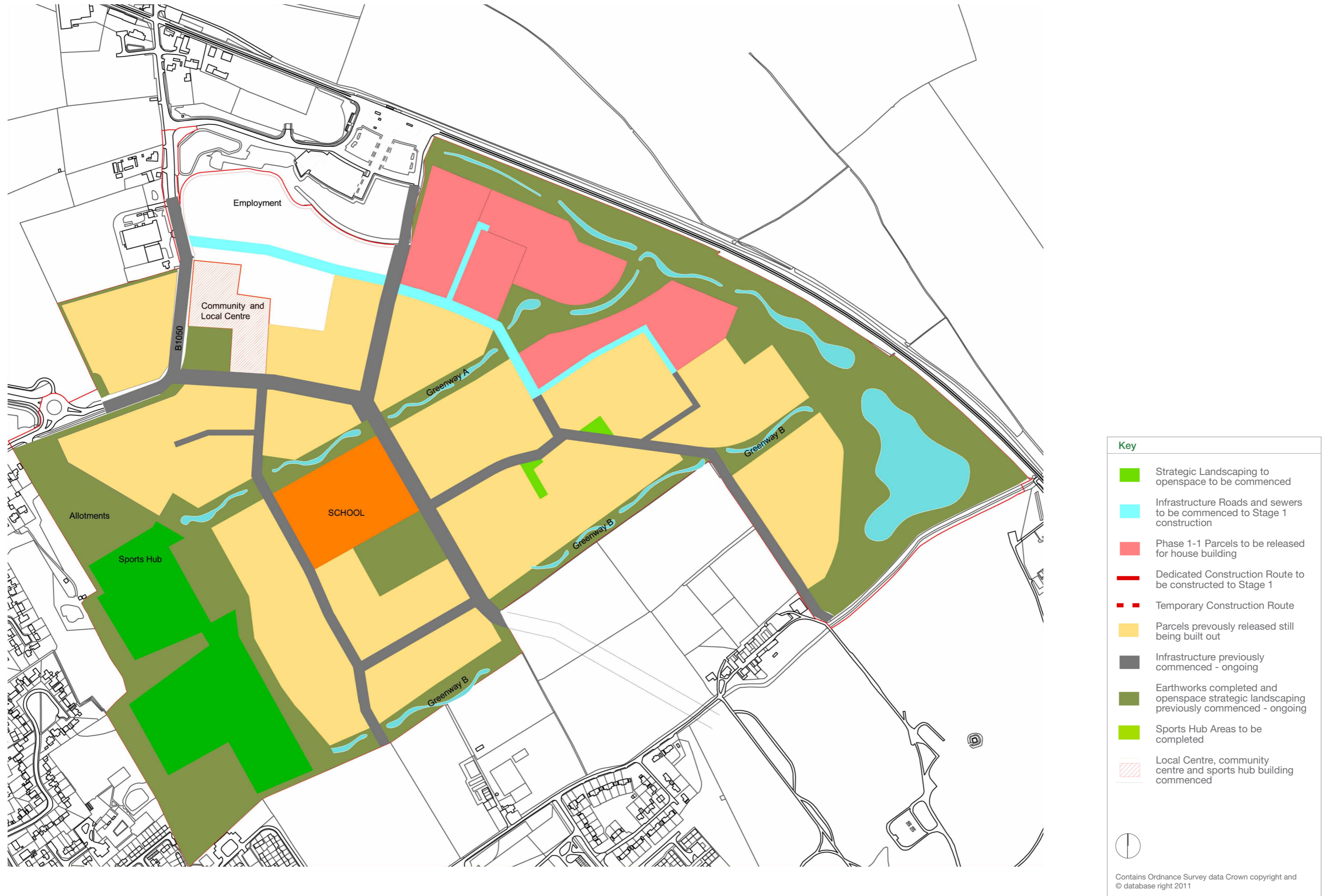
Figure 2.6D Construction phasing: phase 1-4
