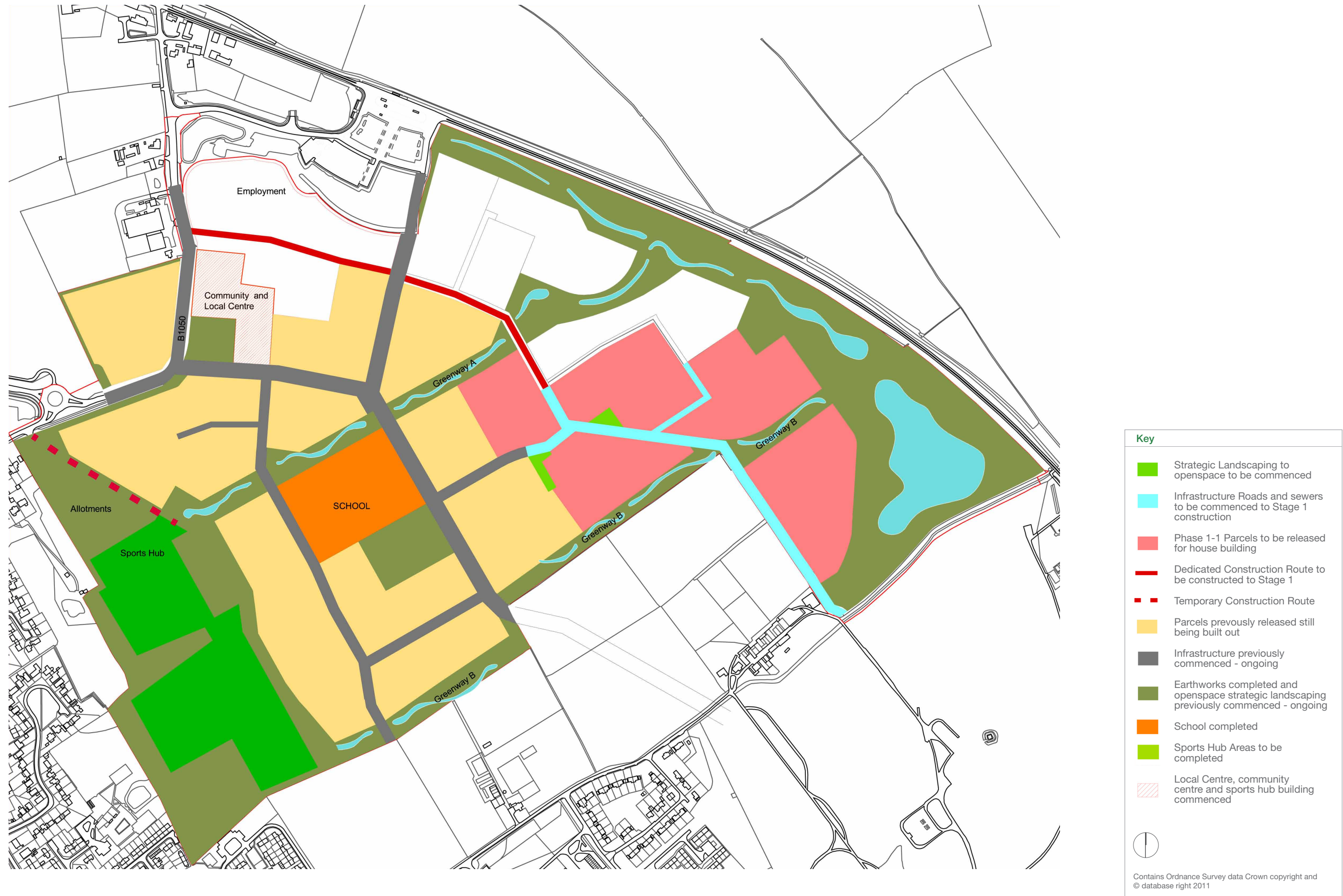
Figure 2.6C Construction phasing: phase 1-3
