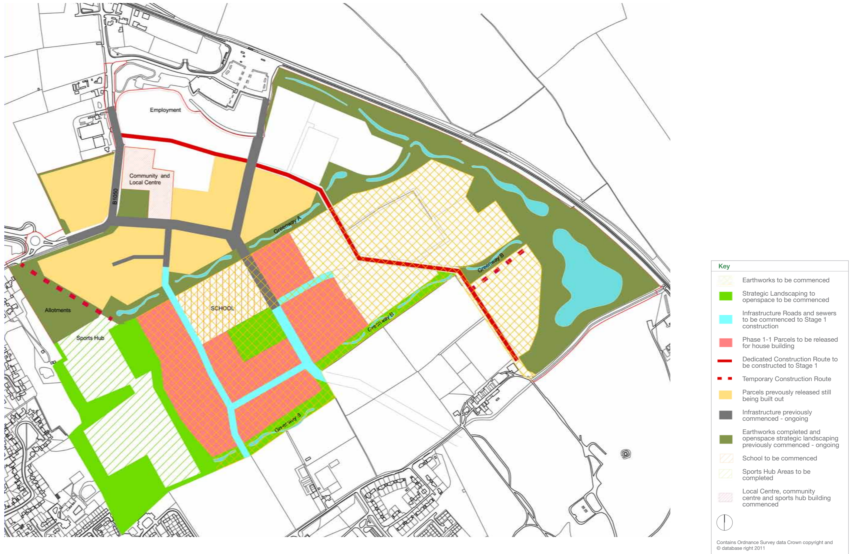
Figure 2.6B Construction phasing: phase 1-2
