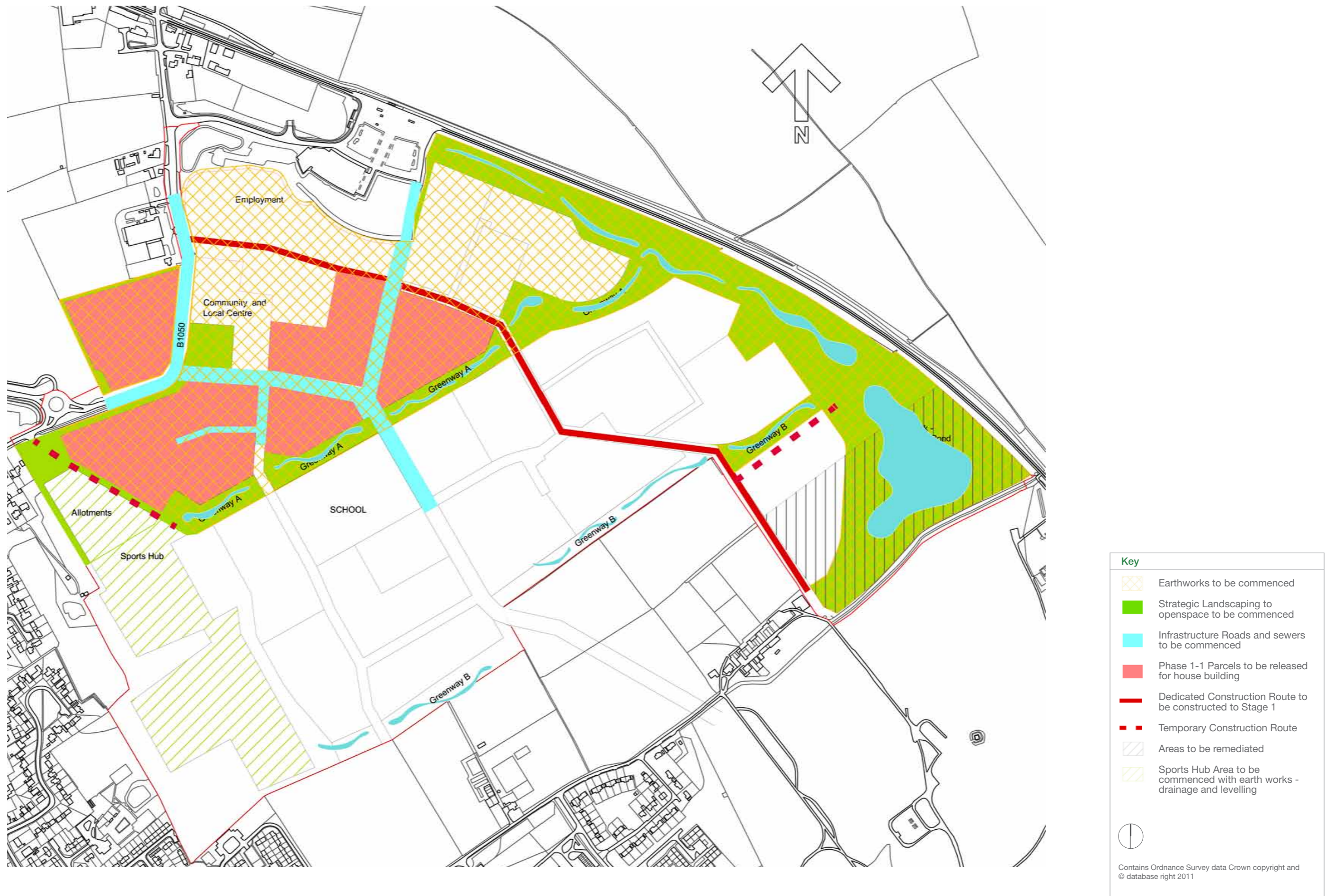
Figure 2.6A Construction phasing: phase 1-1
