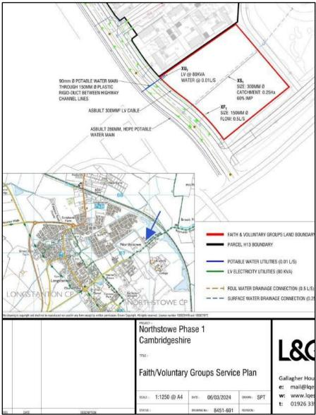
Figure 12: Extract Water Pipe running through the centre of the site
