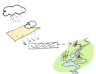
Rainwater harvesting to capture and recycle surface water.
