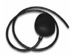
The U bend toilet bung is an example of a simple, inflatable device used to prevent sewage backflow coming back up the toilet under flood conditions. Essentially the U bend toilet bung is a strong rubber bag, attached to a hose with a Schrader valve on the end. The bung is normally supplied with a hand pump.
