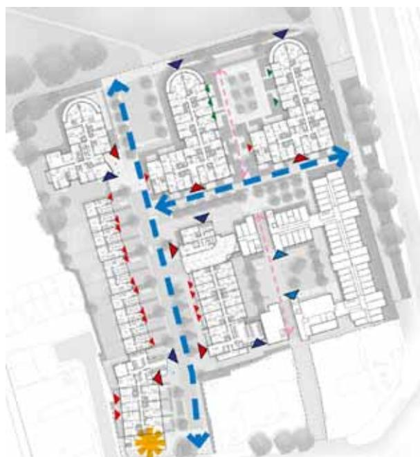
Fig 15: Diagram used to illustrate the movement and connections, for vehicles, cyclists and pedestrians and illustrates the level of ground floor activity, e.g building entrances (John Thompson and Partners, 2009)
