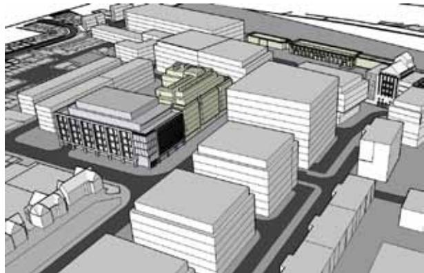
Fig 7: Basic 3D model used to illustrate the scale and massing of a development proposal (Joint Urban Design Team, 2009)
