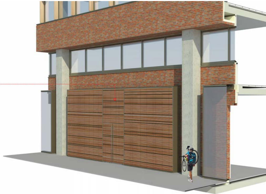
Type 02 - Aluminium Boxed vitrine with Timber BOH facade.
