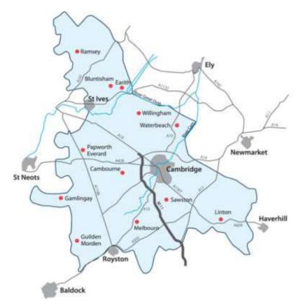
The network comprises five supply zones – the Cambridge zone is the largest of these, in terms of both supply and demand. Sources which supply water direct into this zone provide more water than is needed there to meet demand, so the surplus water is transferred to other zones as required.
