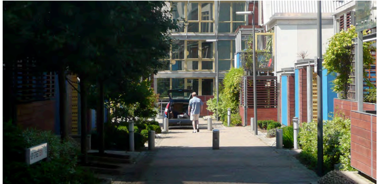
Shared street with bollards to limit vehicle access
