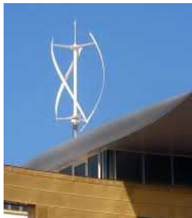
Picture 4: Micro-Wind Turbine (multiple required for reasonable yield)
