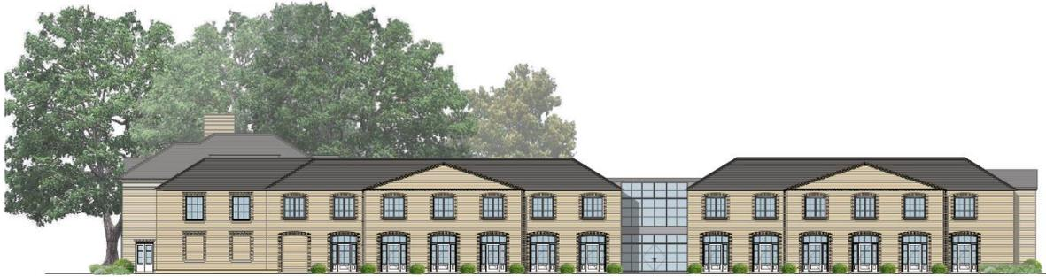
Figure 24 - Northern elevation (Carless + Adams) showing two storey glazed link.
