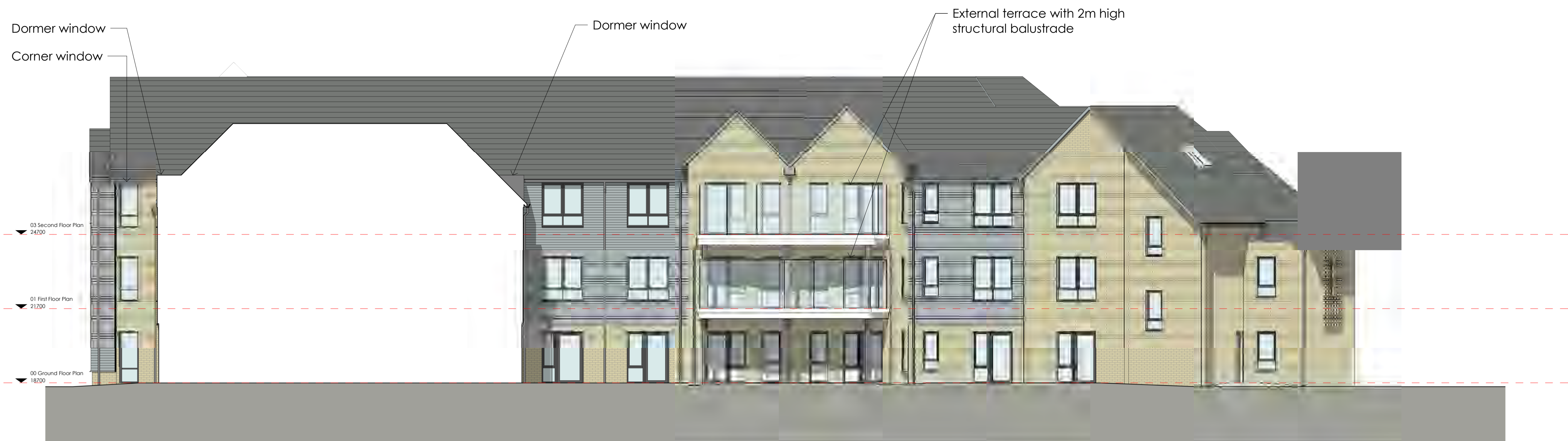
01 WEST SECTIONAL ELEVATION
