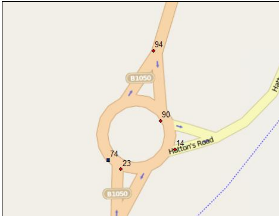
Figure 3.3 – Accident locations at Hatton’s Road / Over Road roundabout
